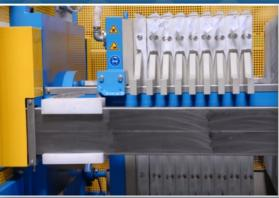
The light barrier or safety grate is installed on our filter presses according to applicable safety regulations.
