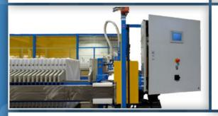
Our automatic filter press is operated through PLC controls. Visualization is done on a key screen or a touch panel.
